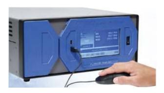
The T series Analyzers from M/s. Teledyne API – USA measure sulfur dioxide, hydrogen sulphide, nitrogen oxides, nitrogen dioxide, ammonia, carbon monoxide, carbon dioxide, and Ozone.
