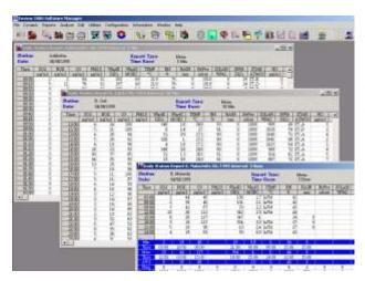
The Data Logger will have the ability to log Channels at different intervals with the capability of averaging and displaying real time data and averaged data over selectable periods (minutes, hours, days, months and years) such as 1 min, 10 min, ½ hr, 1 hr., 4 hrs., 8hrs., 24 hrs., 1 month, 3 months, 6 months, year etc.
