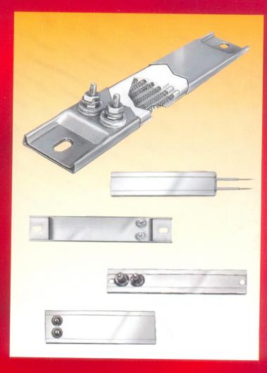
These heaters are also available with fins for air heating applications. The fins have been specially designed to provide maximum surface contact for good heat dissipation thus resulting in rapid heat transfer to the air.
