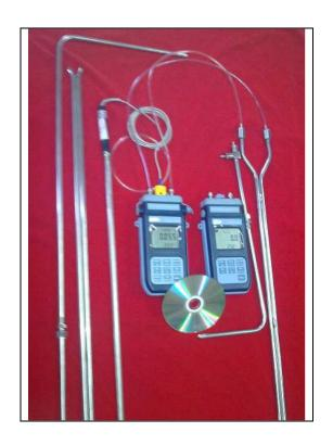
(\*) TC = Pitot tubes with thermocouple K
