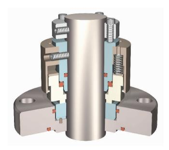
HIFAB dry running single seals type SSDB-E2 can replace conventional gland packing effectively and economically. An innovative seal setting collar simplifies the installation even on large diameter shafts. Hydraulically balanced stationary face is free from any clamping stresses which cause leakage during start-up. The seal can tolerate large radial runout.
