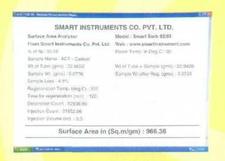
Adsorption / desorption data points are stored and it can be viewed by using Smart Sorb Software.
