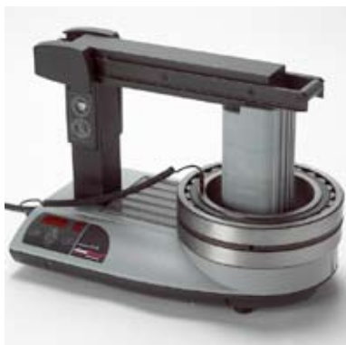
IH 210 with bearing around coil. This position of the bearing guarantees the best efficiency of the heater.
