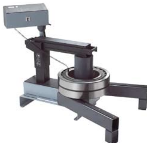
IH 240 with sliding yoke, bearing placed around the coil.
