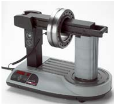
IH 210 with sliding yoke 70 x 70 x 420 mm. Bearing is heated in temperature mode on horizontal yoke.
