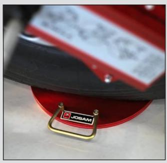
The non-friction plate makes it easier to move the wheels for the toe adjustment and adjust double steering front axles.
