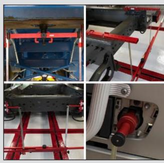
Available with the system are various adapters and brackets which can easily provide extensions to the vehicle.
