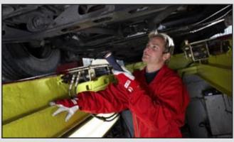
Before measuring wheel angles, the play detectors are used to check for worn parts.
