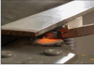
The heat is applied directly to the material being worked on without the necessity for removing heat-sensitive components located in the vicinity.
