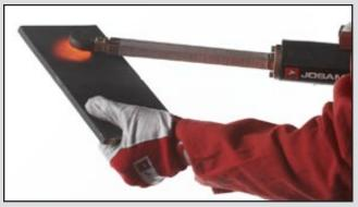
The inductor's round shape makes it possible to achieve unbeatable results, both with heating and shrinking. It can easily be replaced with a completely new inductor or rebuilt by removing the worn out parts, and putting in new parts.
