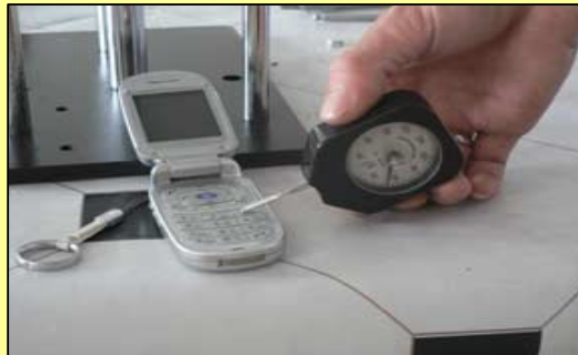
Testing pressing force of push buttons
