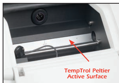
TempTrol heating and cooling Peltier transfer surface
