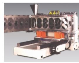
HKC 6/50 with 6 chambers of each 50 I useful volume. Up to 1 t/h of rubber-masterbatch is processed in this CONTERNA. All renowned European masterbatch producers changed over to this continuous production process.
