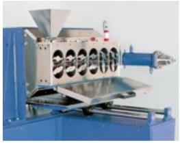
An HKC 6/2,5 with 6 chambers of each 2,5 I useful volume. This size is especially suited for development of recipes, parameter optimization or as a pilot plant. A machine of this size is available for trials in the pilot plant of the IKA\* process equipment division.
