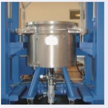
Very easy cleaning of the kneading bowls and – depending on product viscosity – discharge through a bottom outlet valve and under vacuum may save one or several process steps. The product can directly be dosed from the kneading bowl via a transport system into the packing unit.
