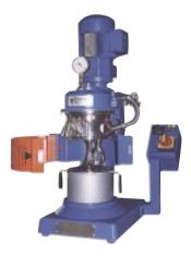
PLANETRON® heavy-duty kneading machines are working with kneading blades that are only one sided running on bearings. Thus the product to be kneaded does neither come into contact with seals nor bearings, resulting in highest product pureness. The use of several kneading bowls enables a semi-automatic process.
