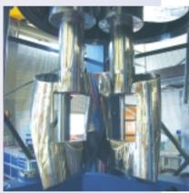
IKA-PLANETRON® vertical kneading machines are available in many different sizes. They can thus be used from research (e.g. development of recipes) with minimum useful volumes starting from 100 ml up to mass production with useful volumes up to 1600 l.
