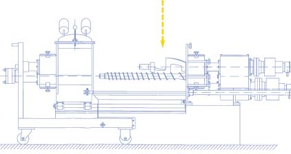
A very large viscosity range from – for a kneading machine – rather low-viscous glues (hotmelts) up to extremely high-viscous rubber mixtures can be processed with the IKA\* horizontal kneading machines with DUPLEX or ZETA blades.
