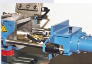
Due to useful options like e.g. discharge screw, removable sidewall or removable kneading bowl IKA® kneaders became the standard machines for many applications.
