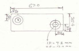
Sketches giving details of front and back connected 20A Fuse fittings
