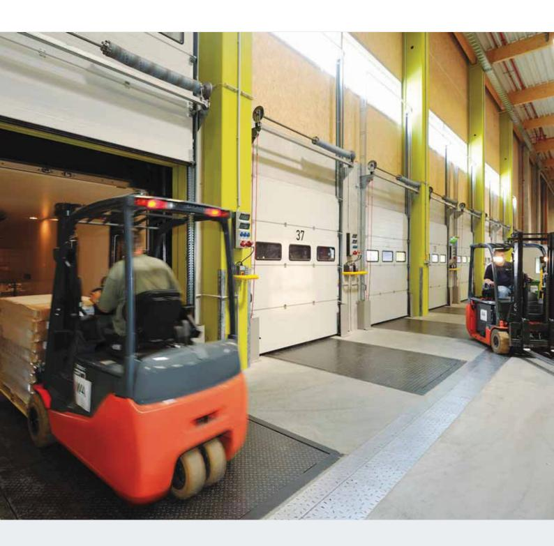
Hydraulic dock levellers are available as hinged lip or telescopic dock levellers. With a length of up to 5 metres, they can bridge large height differences between the ramp and the lorry loading level. Up to a size of  $2000 \times 3000$  mm, the dock leveller platform is made of a single piece. Longer dock levellers are connected by a stable, continuous weld seam. **All Hörmann dock levellers comply with the requirements of EN 1398.**
