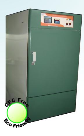
Laboratory Environmental Test Chambers are designed & fabricated to suit Various I. S. standards application in the growing field of Medical, Agricultural, Industrial, Research Laboratories, Metal Treatment & Various Industries. It has a cutting edge technology to challenge & maintain Climatic conditions above freezing what so ever & where ever you need.
