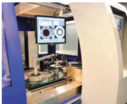
Basler Vario2 fully-automated inspection system
