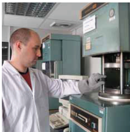
Assessing cure characteristics of mixed compounds by rheometer
