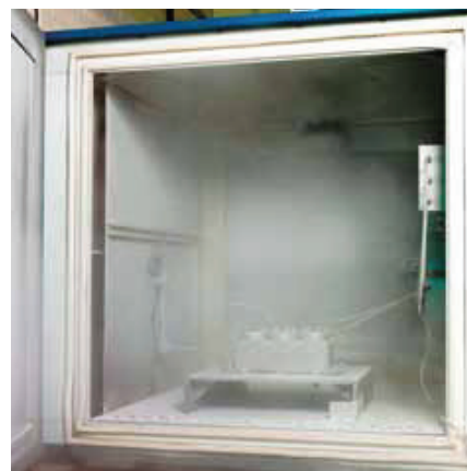
Pressure testing seals at low temperature in 1m 3 (35ft 3 ) environmental chamber
