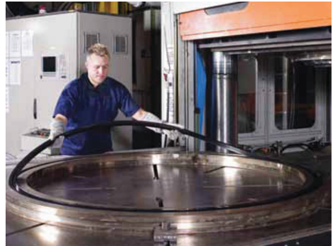
Precision moulding of seals to 2.1m (83 inch) diameter
