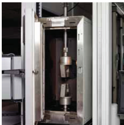
Tensile testing in environmental chamber
