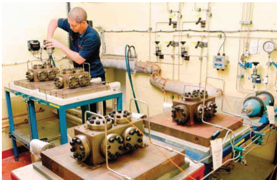
James Walker's eight-flange rapid gas decompression test rigs
