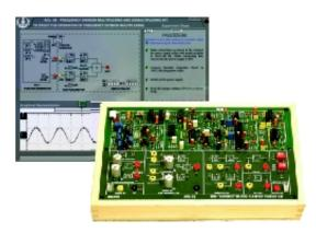
ACL-06 is an analog communication trainer kit designed to study the fundamentals of frequency division multiplexing using DSB modulation technique. Using this module students can well understand the basics of the Balance Modulator, Band Pass Filters, Demodulators and Frequency division multiplexing and demultiplexing techniques.
