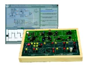
ACL-04 facilitates students to learn a wide variety of frequency demodulator circuits & works with ACL 03.
