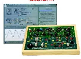
ACL-02 is a Super-heterodyne Receiver with two on-board detectors, an Envelope Detector for Demodulation of Double Side-Band AM signal and a Product Detector for demodulation of Single Side Band AM signal. ACL-02 is capable of receiving and demodulating the Single-Side Band and Double-Side Band signal transmitted from ACL-01. ACL-02 can also receive Double-Side Band AM broadcast signals in the AM wave band.
