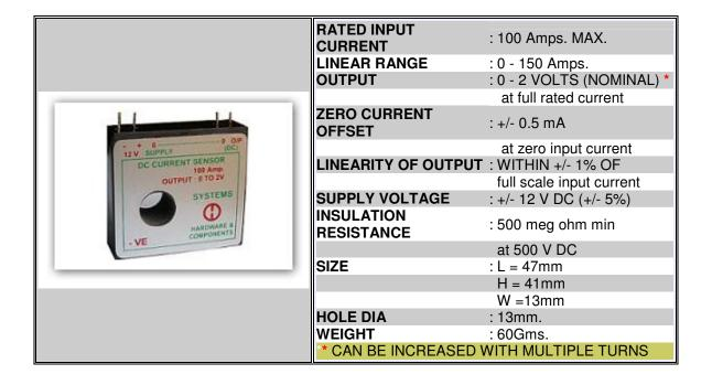
Hall effect Current Sensor gives isolated DC voltage out put proportional to the AC or DC Current passing through. Sensors with higher Current ratings are in the offing.
