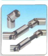
These are manufactured from alloy steel with heat treated working parts, with and without finish bore as per customers requirement. Available up to 8" Od and up to 4" shaft size and 2000 kgm Torque.
