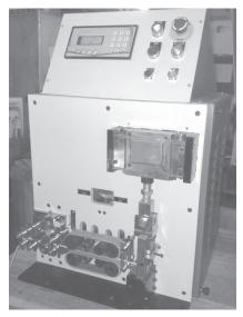
This power-packed machine ensures high production volumes and low manufacturing costs. With these machines, the cost of cable cutting is around 10 to 15 paisa per 100 cables. A stepper motor drive and an encoder feedback system ensure high accuracy in length. Machine being accurate, it saves copper and often the saving in copper cost is much more than the labour saving. Most importantly, this machine does not require any compressor, and can be operated with single-phase electric supply.
