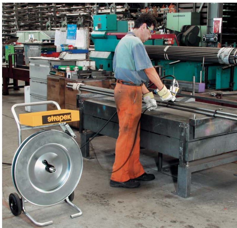
Model STA 76 for oscillating wound steel strap
