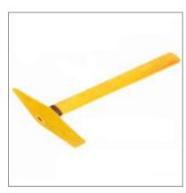
475gms Anti-Spark Chipping Hammer is used in area where chipping sparks are not desirable like oil industry. The Chipping Hammer is designed with an anti-spark brass head and wooden handle that facilitate ease of operation. The Chipping Hammer is available in a weight range of 475gms and in 280mm length. 475gms Anti-Spark Chipping Hammer is used as a welding tool and comes under CHWH-Brass model.
