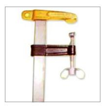
600 Ampere Current Operated F Clamp has a throat depth of 63.00mm and is offered in 982gms weight range. The F Clamp is equipped with a brass jaw that facilitates ease of operation. The F Clamp can operate using 600 Ampere current and used for welding purpose. 600 Ampere Current Operated F Clamp is designed with a clamping gap of 170.00mm and comes under ECF60NB model.
