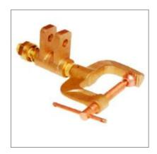
Heavy Duty Rotary Ground Clamp with Brass Body is available in a range for 500 Amps to 1000 Amps. The Rotary Ground Clamp delivers efficient grounding of rotating object and ensures easy connectivity to welding fixture. The Rotary Ground Clamp of model number ECR 1000-2 is available with one/ two cable connectivity facility. Heavy Duty Rotary Ground Clamp with Brass Body comes with tension spring to ensure maximum contact between conducting surfaces.
