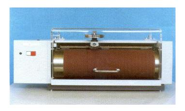
The Abrasion Tester is used to evaluate the resistance of elastomers to frictional wearing Abrasion tests to this testing standard are performed on samples of materials which undergo wear and abrasion during their normal working life (e.g. tyres, conveyor and drive belts, shoe soles).
