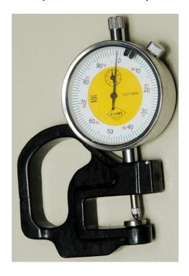
Suitable for checking various materials in production control, routine and series test available in different range accuracy and throat as per Standards specification. Sample Thickness 0.01mm to 10 mm.
