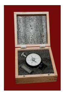
The Shore Hardness is defined as the resistance to penetration by an indentor of specified shape under a defined load.
